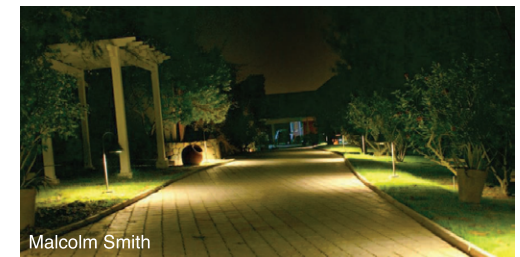
Malcolm Smith This fully shielded lighting with motion sensors safely light the walkway and saves energy.
