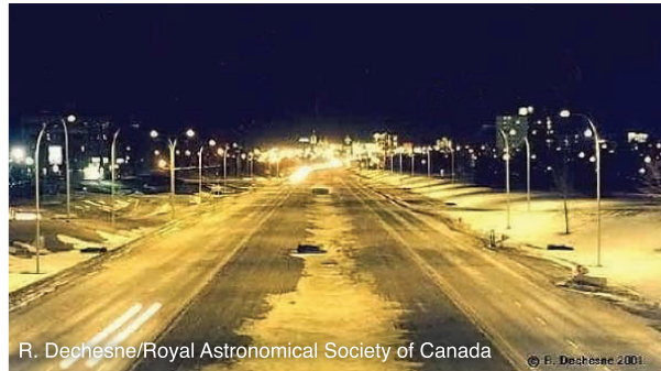
R. Dechesne/Royal Astronomical Society of Canada © F. Dechesne 2001 Notice the glare of the old drop lens fixtures in the background compared to the new flat-lens fixtures in foreground, Calgary, Alberta, Canada.
