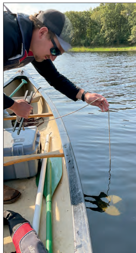
Above: Colton Sorensen, Polk County Land & Water Resources Dept. lowers a secchi disc into the water to measure water clarity. Note: remove sunglasses before taking a reading.
